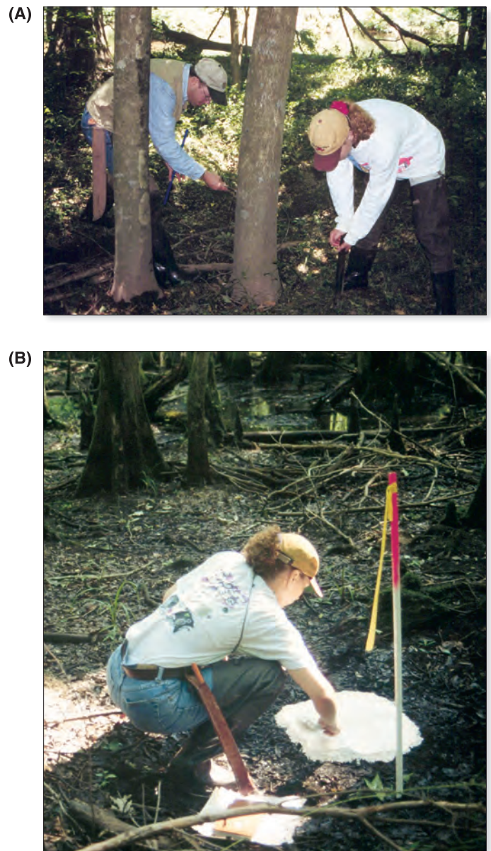
Figure 7. (A) Dendrogeomorphic and (B) clay pad techniques, long and short term, respectively, for estimation of sediment deposition rates. [(A) shows one person coring a tree for age determination and another probing for depth of root burial. (B) demonstrates the placement of the white feldspar clay pads on the flood-plain surface.] Photographs by Cliff R. Hupp, U.S. Geological Survey.
